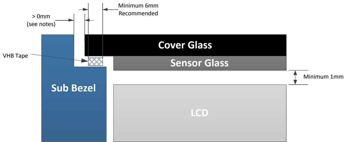
Figure 2-2. Standard Integration of a PCAP Touchscreen with Bezel (not to scale)
