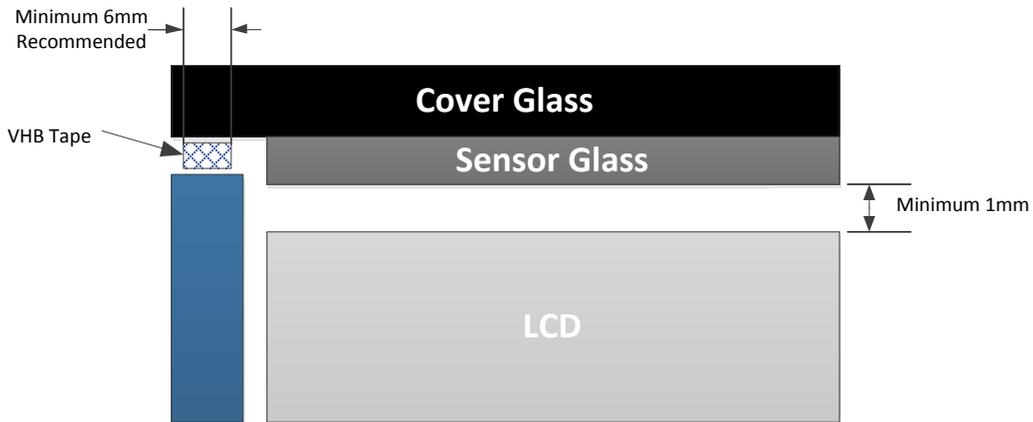
Figure 2-3. Standard Integration of a PCAP Touchscreen without Bezel (not to scale)
