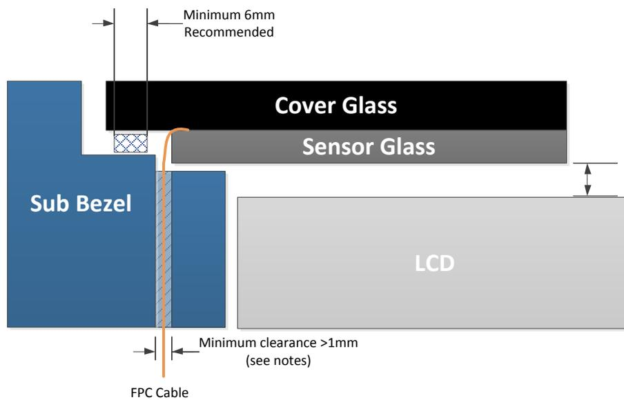
Figure 2-4. Standard Integration with Slotted Sub-bezel (not to scale)
